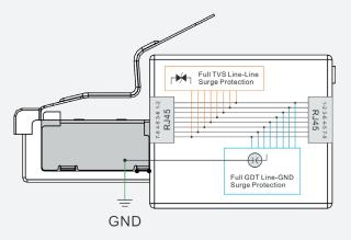
**Note:** The metal release tab does not provide a ground connection. Ground connection is made by connection with the metal sides as shown in grey in the diagram with green GND connection.
